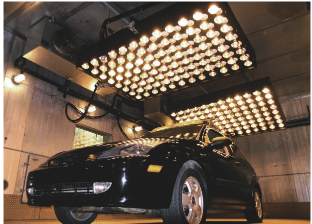
Over 45 kW of heat penetrate down on the top of a vehicle during an infrared heating test within a drive test chamber.
