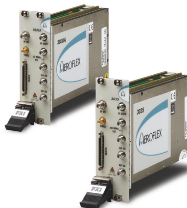
The 3030A digitizer operates from 330 MHz to 3 GHz with a 33-MHz digitized bandwidth, while the companion 3035 operates to 6 GHz with a 36-MHz digitized bandwidth.
